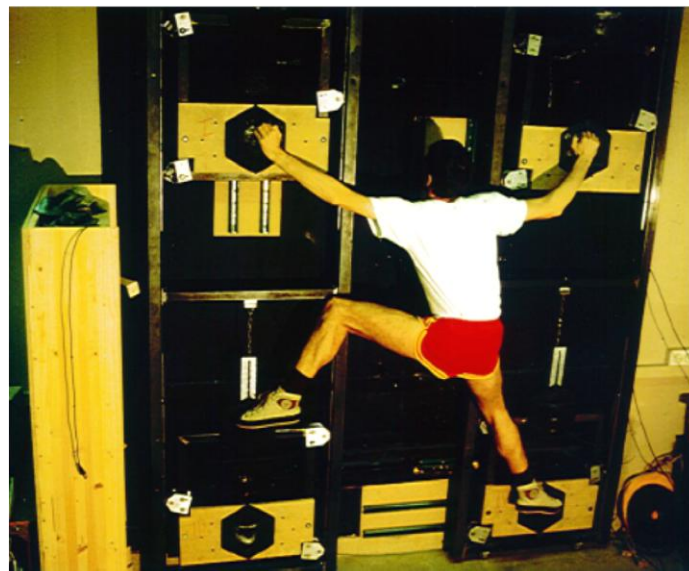
Figure 1 –Patrice Rougier at work on the first equipped climbing wall in Grenoble University. Each hold was equipped with 1D-vertical force sensor
