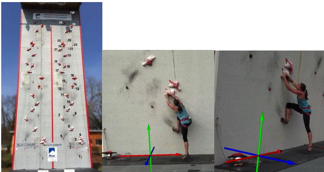
Figure 1 - The official speed climbing wall - 3D reference frame calibrated and the hip marker on the harness.
